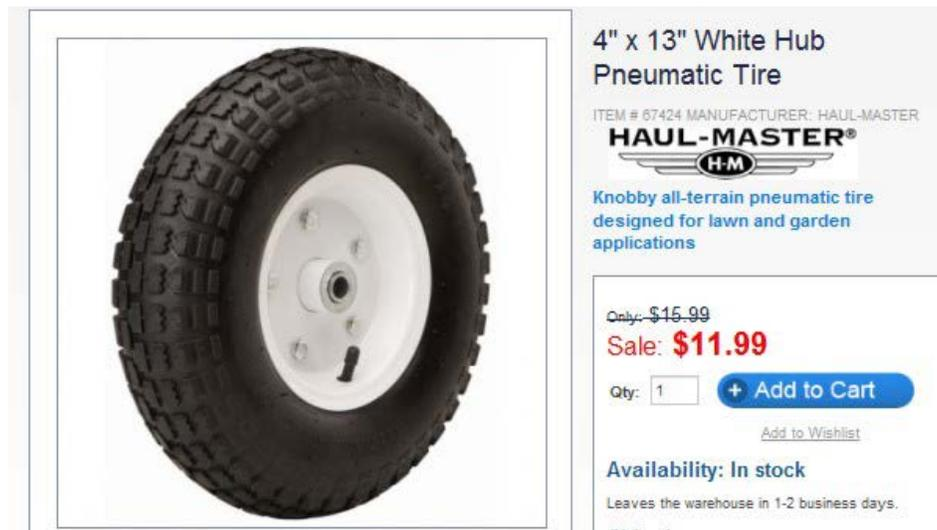
Wheels fit on a 5/8" axle. A 5/8" bolt 4-1/2" long is just the right size to go through the hub. Wheels must have some sort of locking arrangement on the nut such as a locknut or an additional nut.
