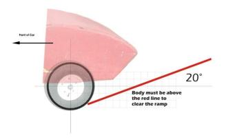
Car must have 4 wheels and all four wheels must be in contact with the track at all times.
